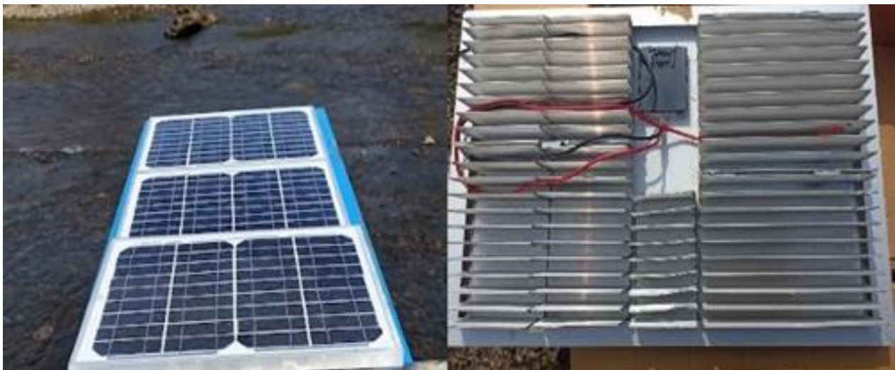
Figure 2. Monocrystalline Solar Panels with Heatsnik Cooling Fan
