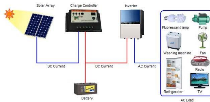
Gambar 1. Skema Solar Home System (SHS)[4].
