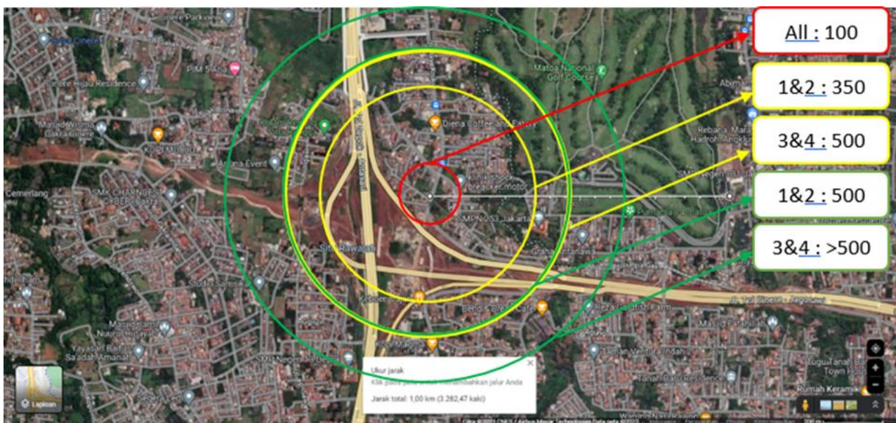
Figure 5 Threat zona of overpressure
