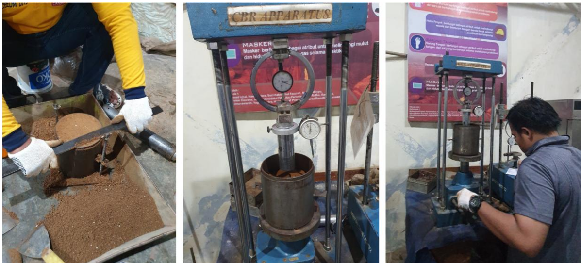
Figure 6 . CBR test at the laboratory
