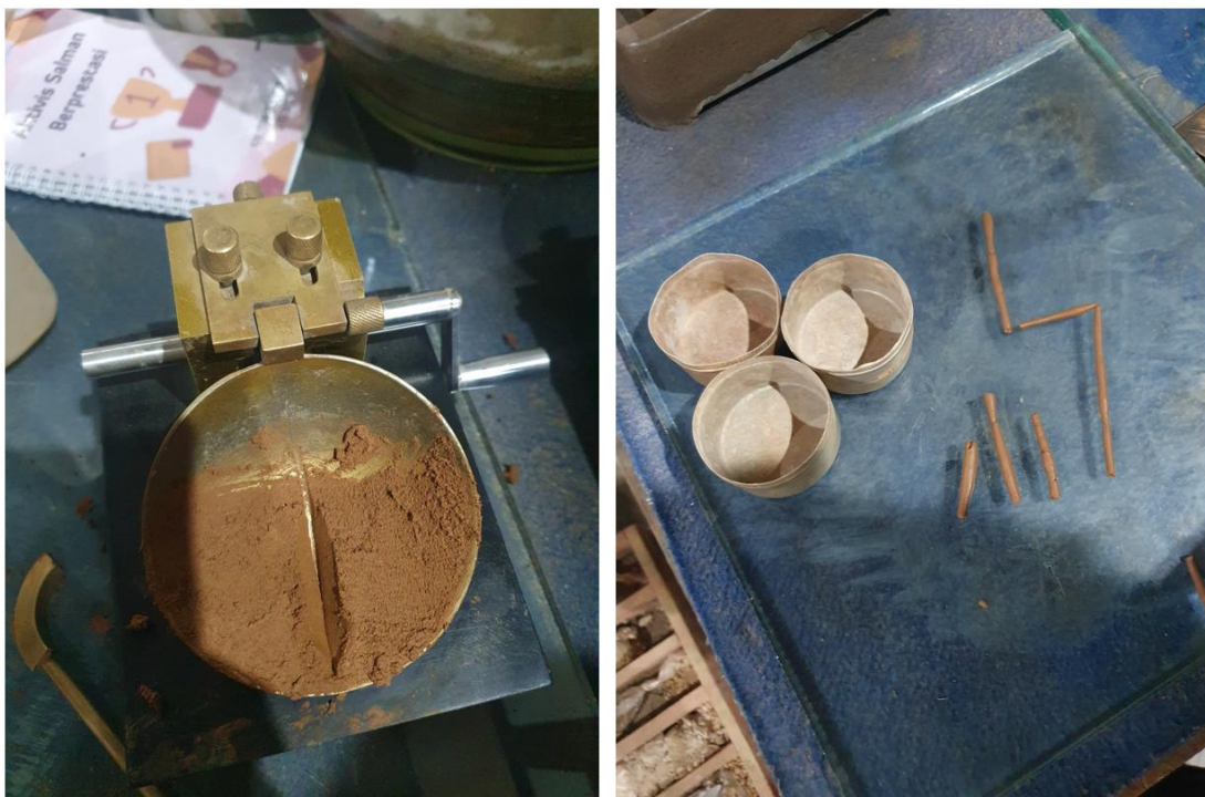
Figure 5. Liquid limit and plastic limit test
