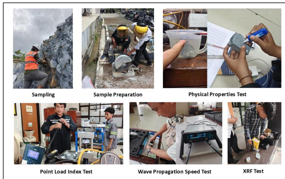
Figure 5. Rock Sampling and Laboratory Testing of Rock Samples
