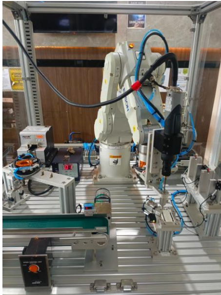
Figure 7. Robot movement to screwing station
