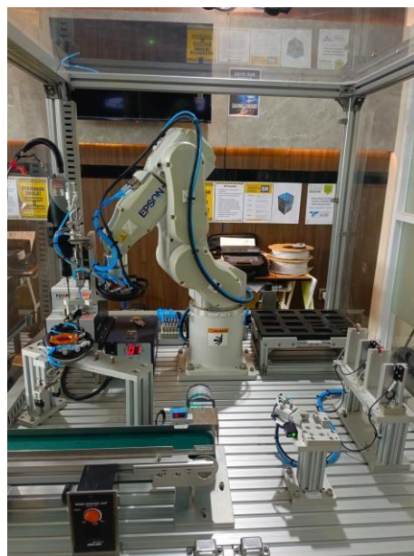
Figure 6. Robot movement to screw feeder
