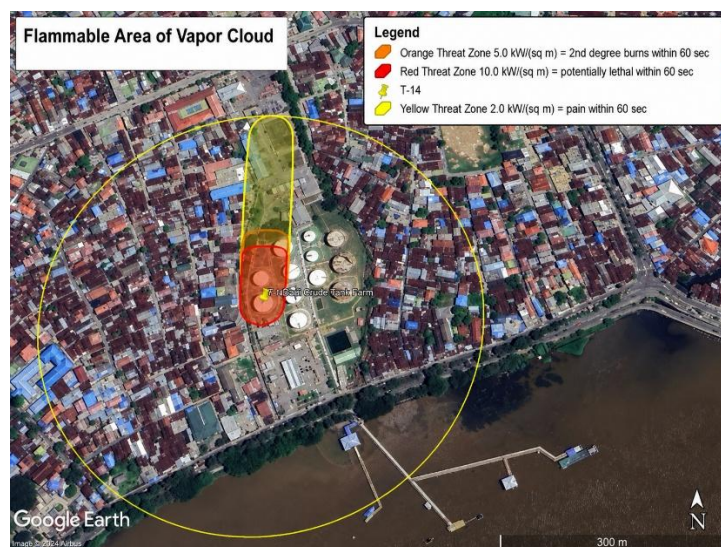
Figure 4. Pool-fire thermal radiation threat zones for the modeled gasoline overfill scenario.
